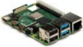
A photograph of a Raspberry Pi model B, a small green single-board computer with various ports and components visible.                                        |
