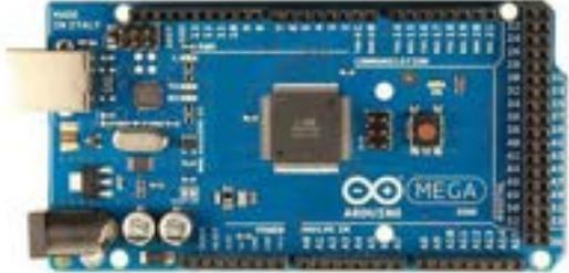
A photograph of an Arduino Mega microcontroller board, which is blue and features a large ATmega2560 microcontroller, a USB Type-B port, and several headers. |
