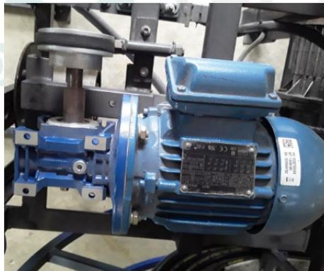
Figura 8 - Motor reductor.
